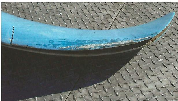
*A cracked-up fibreglass impeller*
